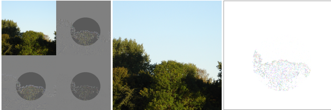
Figure 7: Left: Decomposed image with capacity maps overlaid. Center: Watermarked image. Bits_{min} = 1 and Bits_{max} = 3 yield an average encoded bit rate of 2.77 bits/pixel (total number of encoded bits: 130209). Right: Scaled difference between original and watermarked image (the darker a pixel value, the higher the difference).
