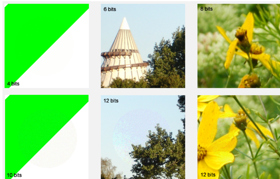
Figure 12: Image parts which were watermarked using the LSB technique. The upper row shows evaluated images which have the lowest amount of data encoded, the lower row shows images with the highest data amount encoded. The circular region, into which the watermark stream was inserted, is located in the center of an image.
