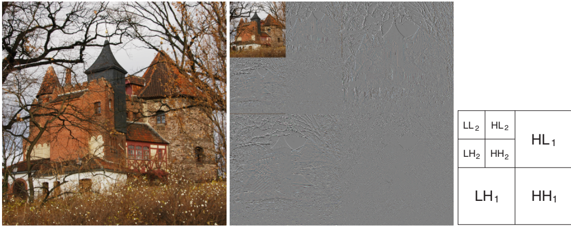
Figure 5: The original image (left) is wavelet transformed using a 2-level decomposition (middle). The transformation results in low-, middle-, and high-frequency subbands ( LL , HL , LH , and HH ).
