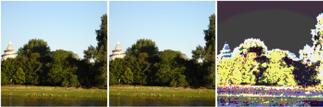
Figure 3: The original image (left) has been watermarked (center) according to the determined capacity map (right). On average, 7.8 bits were encoded per pixel; in terms of each individual color channel, 2.7 bits (red), 2.66 bits (green), and 2.5 bits (blue) were embedded.
